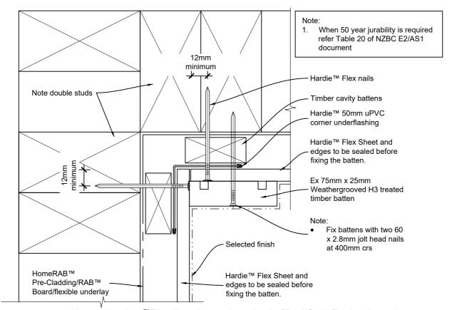
Alternatively an Axent™ Trim with two 6mm continuous beads of Bostik Seal n Flex-1 can be used
